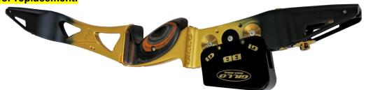
Assembling Heavy weight Bare Bow covers over the G2 is not suggested as the four M4 threaded holes of G2 can't support them properly. Damages coming form use of heavy covers on the G2 will void riser warranty. Please refer to the specification sheet of the various covers to check if they are suitable for the G2 riser.
